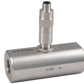
Fluid flowing through FTB200 causes the rotor to revolve. As the rotor blade pass the pickoffs, electrical pulses are produced in which frequency is proportional to the flow rate. The revolutions per minute and the K-factor (number of pulses/Gallon) make it possible to obtain the flow volume passing through the unit.
